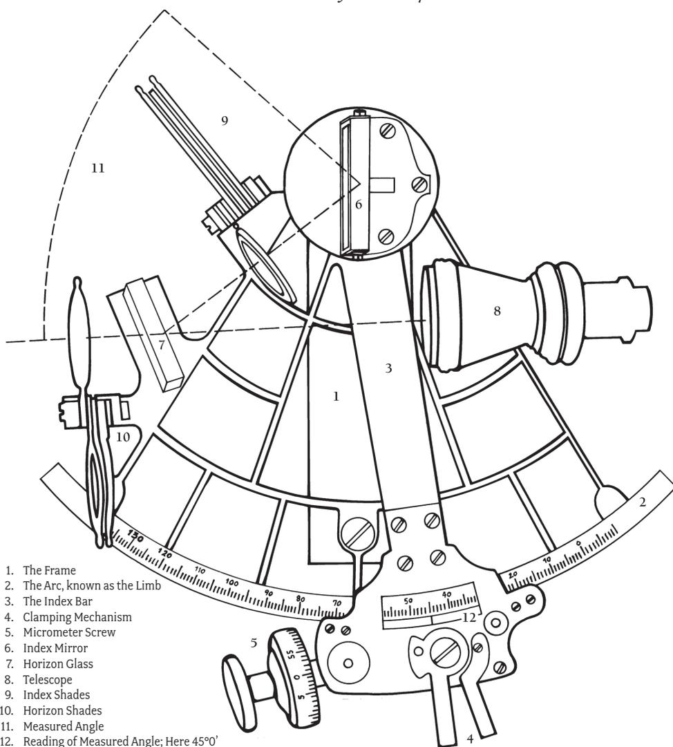
For the sun or moon, the upper or lower limb (or edge) of the object should be exactly at the horizon. For a star or planet, it should be centered on the horizon line. Now rock the sextant back and forth a few times to see that the object has been measured at its lowest point. This check will assure that the sextant is perfectly vertical. When you're satisfied with the sight, note the exact time, and read the elevation from the arc and micrometer drum or vernier scale.
